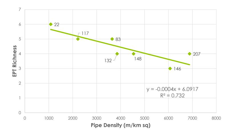
Relationship between the pipe density (meters of pipe per square kilometer of land) and EPT richness (stream health index based on macroinvertebrate data) for seven watersheds in the North Carolina Piedmont.
